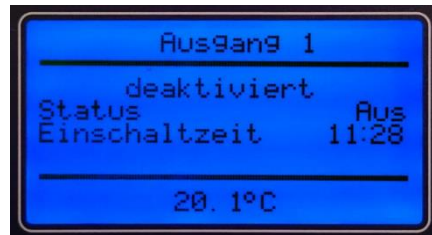
Fig. 3: Display of the output port status.
