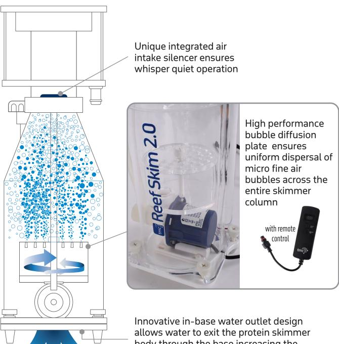
Innovative in-base water outlet design allows water to exit the protein skimmer body through the base increasing the air-water contact time within the skimmer and reducing both noise and the amount of micro bubbles escaping the body.
