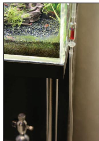
Unscrew the hosetail locking nut on the pressure regulator and then thread the other end of the flexible CO<sub>2</sub> tubing into the hole in the end of the locking nut, and attach this same end to the outlet hosetail. Re-attach and secure the hosetail locking nut.
