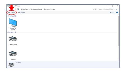
d. Select the MCU from the displayed options in the "Add a device" popup screen (it should be identifiable by its serial number which should match the number printed on the outer label of the unit)
