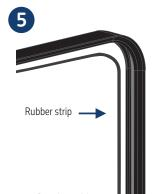
Cut the rubber strip to length, then push it into the cable channel so it completely covers and holds the cable in place.
