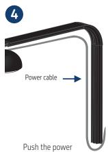
Push the power cable exiting the light unit into the cable channel in the underside of the 90° arm fitting.
